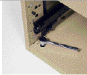
Use a 1/4" socket wrench to adjust glides from inside. The glides allow adjusting from inside or outside and allow accurate leveling of the cabinet.
