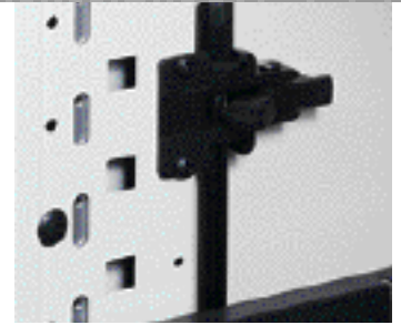
Laterals feature the Series XXI patented interlock. The interlock promotes safety by preventing more than one drawer from opening at a time. By automatically restaging, the interlock also prevents damage to the system if the drawers are removed and reinstalled.
